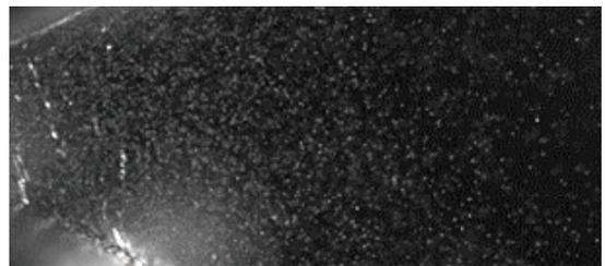
FEA creates spherical monodisperse drops from solutions of Polyethylene Oxide (PEO)"
