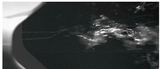
Conventional atomizers create poor quality spray with filaments and irregular droplets from solutions of Polyethylene Oxide (PEO)"
